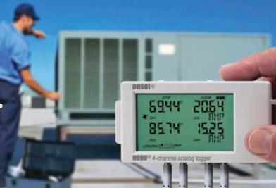
**ACCURATE TRACKING** The new HOBO UX120-006M Analog Logger for buildingperformance monitoring applications provides twice the accuracy of previous models. It features a deployment-friendly LCD, and support for up to four external sensors for measuring temperature, current, CO<sub>2</sub>, voltage and more.
