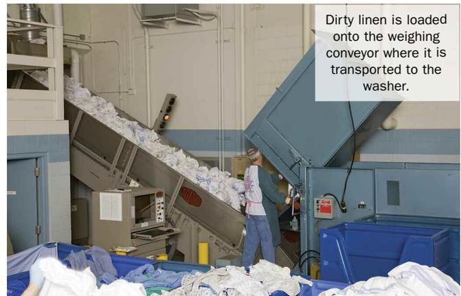
Dirty linen is loaded onto the weighing conveyor where it is transported to the washer.
