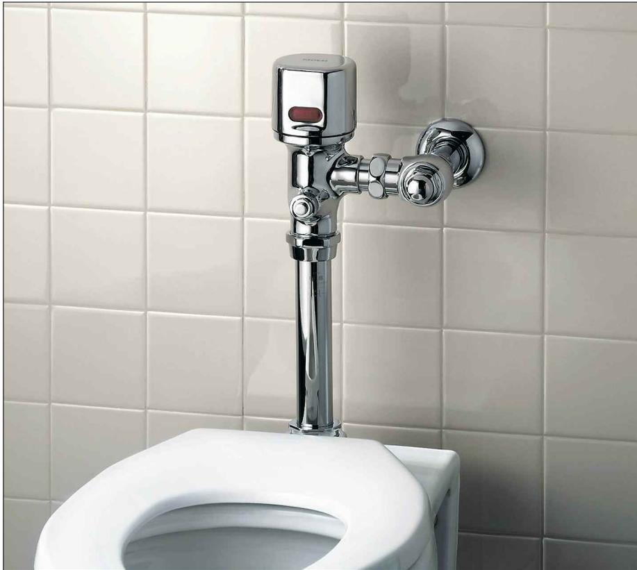
**NO HANDS!** The M•Power high-efficiency flush valve promotes water and energy savings and provides sanitary protection by using an infrared sensor beam to activate a flush cycle when a user leaves its range. It features a flow rate of 1.28 gallons per minute (gpm), a 20 percent savings from the industry standard 1.6 gpm.
