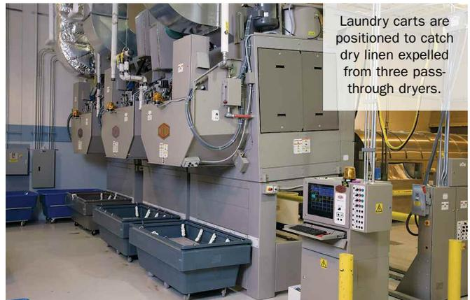
Laundry carts are positioned to catch dry linen expelled from three pass-through dryers.
