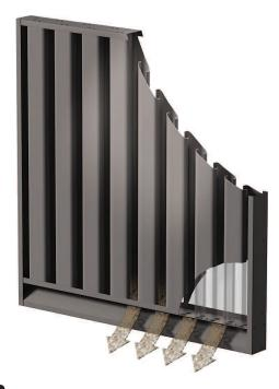
**SAND AWAY** The Model FSL-401 sand louver is designed to protect air intake and exhaust openings in building exterior walls from wind-driven sand. It incorporates vertical sightproof blades to separate sand from the airstream and channel it out.
