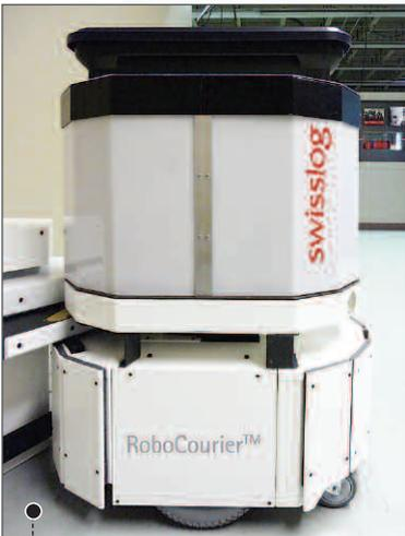
**SPECIAL DELIVERY** The Robocourier autonomous mobile robot can carry and deliver up to 100 pounds. A laser guidance system assures obstacle avoidance and staff safety. It is equipped with preprogrammed destination buttons and battery power.
