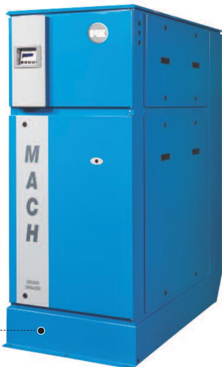
**FLEXIBLE SYSTEM** The new P-K MACH dual-fuel condensing boiler can be changed from natural gas to propane simply by flipping a switch. It features a variable-speed combustion blower and dual modulating gas safety shutoff valve.
