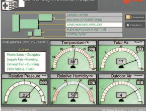
**DRIVING TOWARD EFFICIENCY** The Critical Hospital Systems Dashboard turns a building's automation system into a powerful tool specifically designed for reporting and tracking the needs of health care facilities.
