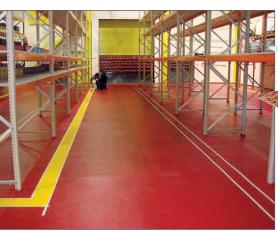
**GETTING FLOORED** FastFloor is a two-component, rapid-curing, hybrid polyurea coating system that protects against abrasions, chemicals and heavy foot traffic. The coating can be applied with a roller or brush and allows return to service within 24 hours.
