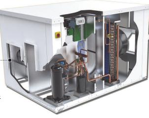
**IAQ SOLUTION** The Reznor Z-series hybrid ventilation unit integrates an energy-recovery wheel into a dedicated heat-pump system for precise ventilation and temperature control. It can recover more than 80 percent of exhaust air. **Thomas & Betts Corp. • www.tnb.com**
