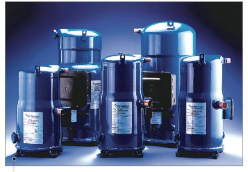
**VERSATILE SERIES** The Performer series of scroll compressors is designed for commercial and light-commercial applications for use with R-410A, R-134a, R-407C and R-22. They are offered in fixed and variable-speed models and in a capacity range of 7.5-30 tons. The series is available in tandem/trio configurations up to 60-90 tons. **Danfoss • www.danfoss.com**
