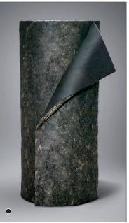
**DUAL ACTION** ToughGard T Textile Duct Liner is an acoustical liner for HVAC sheet metal ducts, improving the energy efficiency of the system by reducing heat gain or loss and minimizing moisture problems due to condensation. Moisture beads up when it enters a duct system with the liner and evaporates before it is absorbed. **CertainTeed**
