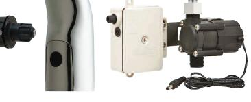
**ENERGY GENERATOR** The faucet's Self-Sustaining Power System features an energy-efficient turbine power option. The SSPS uses turbine technology to create and store power every time it is used. A magnetic dual-inductor rotor turbine creates energy from water flow. Chicago Faucets Company • www.chicagofaucets.com
