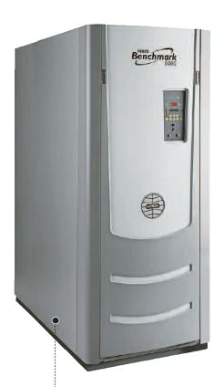
**COMPACT UNIT** The stainless steel Benchmark 6000 boiler features 15-to-1 turndown for energy efficiency and low NOx emissions. The unit has an operating efficiency of 92.5 percent and measures 79 inches high by 34 inches wide by 109 inches deep. A remote data collection option is available.
