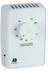
UNDER CONTROL The new CA Title 24-compliant model DS-2080 humidistat sensor controls bathroom exhaust fans based on the moisture levels in a room. The surface-mounted wall control allows the humidity settings to be adjusted from 20 to 80 percent relative humidity.
