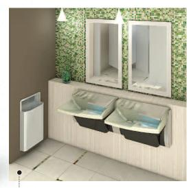
**ALL-IN-ONE SYSTEM** The Advocate AV-Series Lavatory System provides a sink, soap, faucet and dual-sided hand dryer in one unit. Users move their hands from left to right, beginning with a touchless soap dispenser, a touchless 0.38-gpm infrared faucet and finishing with a high-efficiency, dual-sided hand dryer.
