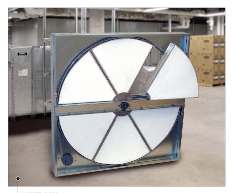
WHEEL DEAL Field-assembled cassettes reduce installation times and costs when replacing large, energy-recovery ventilation wheels. Cassettes are factory-built, tested, marked for reassembly, and then disassembled for shipment. It recycles up to 80 percent of heating and cooling energy in exhaust air. Airxchange • www.airxchange.com
