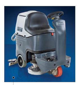
EASY RIDER The SC3000 compact rider scrubber features a 26-inch cleaning path and patented scrub deck. It provides user-friendly, maneuverable operation in multiple cleaning areas, including those with limited access or tight corners. Onetouch Quiet Mode operation allows use in noise-sensitive areas. The EcoFlex System permits easy control of water, detergent and energy.
