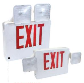
**CLEAR MESSAGE** The new EECLA-R fixture features an exit sign with two adjustable emergency lights that can be positioned at the top of the sign or realigned to either side. Constructed from heavy-duty, impact-resistant thermoplastic, the unit includes two 5.4-watt DC 5 wedge-based incandescent lamps in the emergency light and a 1-watt LED lamp in the sign for energy savings.
