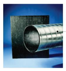
KEEPING IT QUIET ToughGard Ultra\*Round is a fiberglass duct liner overlaid with a durable, fire-resistant black-composite, air-stream surface, which is scored for easy installation in spiral air ducts. The liner helps to absorb equipment and air-rush noise over a broad spectrum of sound by trapping and dissipating it within the glass fiber matrix. It contains an EPA-registered antimicrobial agent.
