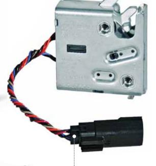
**HEAVY DUTY** Featuring corrosion-resistant plated steel. stainless steel construction and fully-sealed internal actuator, the R4-EM outdoor unit provides reliable electronic locking for outdoor applications. The embedded electronic control allows for easy integration with an external control system, and flexible, concealed installation provides vandal-resistant design.
