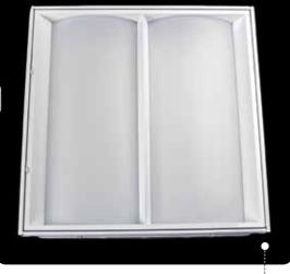
LONG LIFE A new 44-watt, 2 by 2 LED troffer luminaire features curved diffusers, a color temperature of about 4000K and minimum 50,000-hour life. The UL-approved troffer is designed for installation in standard 15/16-inch, T-bar grid ceilings. Two strips of surface-mounted LEDs generate more than 3,220 lumens of light.
