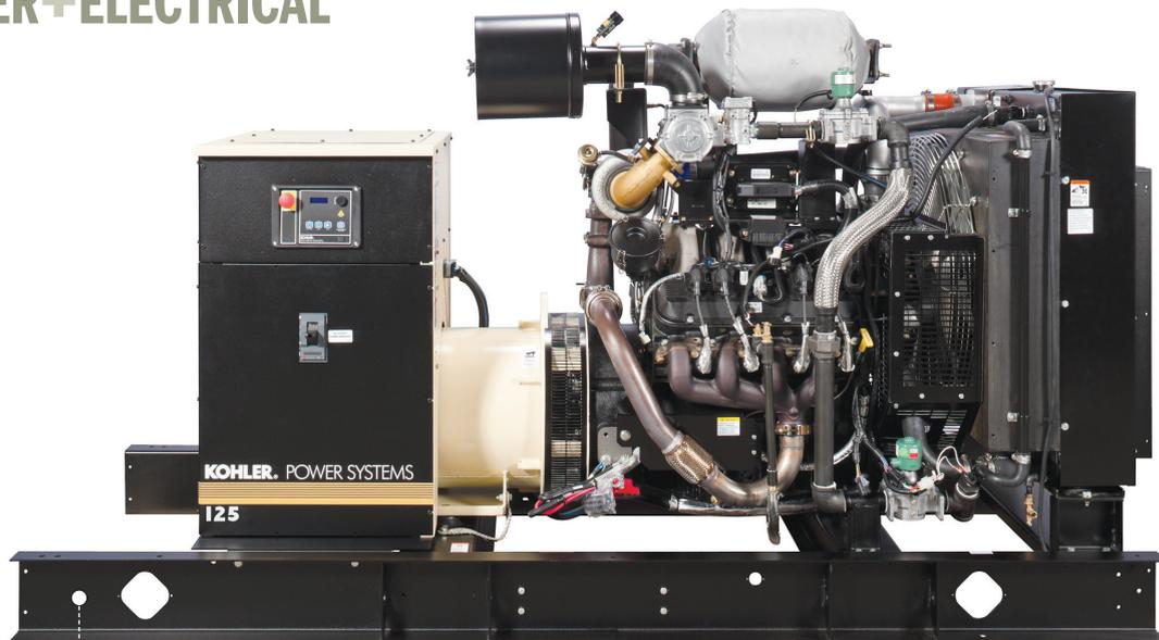
**RELIABLE POWER** The generator set starts within 10 seconds per National Fire Protection Association (NFPA) 110 requirements. The unit and its components are factory-built and production-tested. It operates on a variety of fuel sources, including diesel, natural or LP gas. The 60 Hz unit meets NFPA 110 Level 1 performance standards. **Kinsley Power Systems** • [www.kinsley-group.com](http://www.kinsley-group.com)
