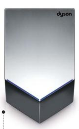
QUICK DRY The Airblade V hand dryer is 60 percent smaller than the original, yet dries hands fast. Two sheets of unheated high-velocity air angled at 115 degrees span the width of each hand and dry hands in 12 seconds. The unit features a brushless DC motor with digital pulse technology for fast acceleration.
