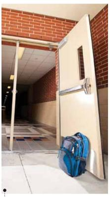
**DOOR GUARD** The battery-powered alarm system guards against propping doors open and assures that doors left open by mistake won't defeat the security system. The EAX-300 Door Prop Alarm can be field-set for door prop times ranging from 1 second to 4 minutes, with a 15-second default. After the time selected, a 100-decibel alarm alerts staff, then silences when the door is closed.
